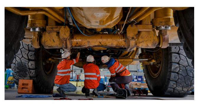
Mobile maintenance employees carrying out an inspection on the underside of a Cat® 777D—100 tonne rigid chassis dump truck at the Phu Kham Copper-Gold Operation.
