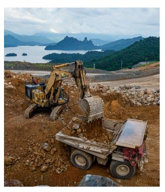
Cat® 777D—100 tonne rigid chassis dump truck being loaded at the Ban Houavxai Gold-Silver Operation.
