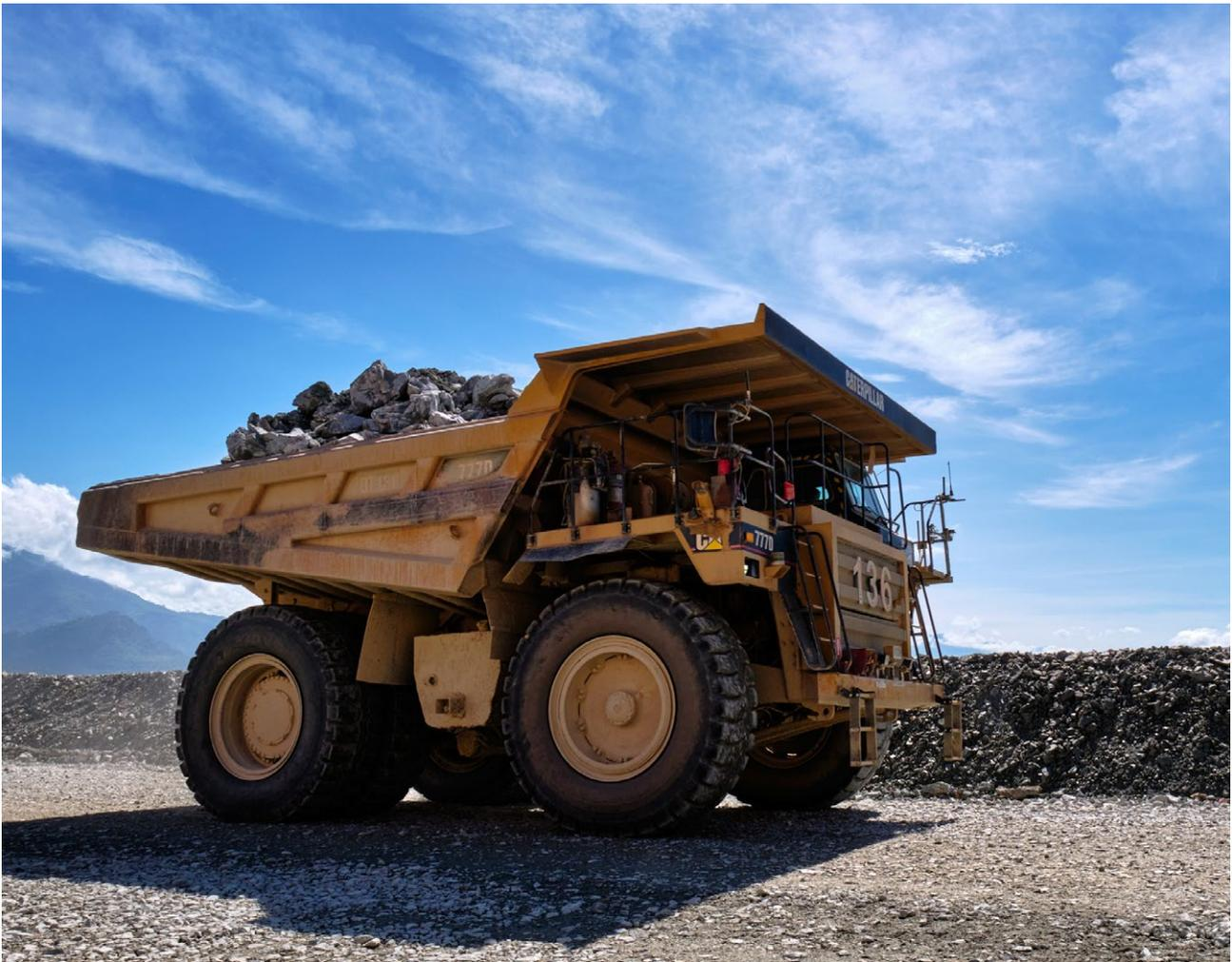
Cat® 777D—100 tonne rigid chassis dump truck fully loaded with ore ascending the haul road at the Ban Houayxai Gold-Silver Operation
