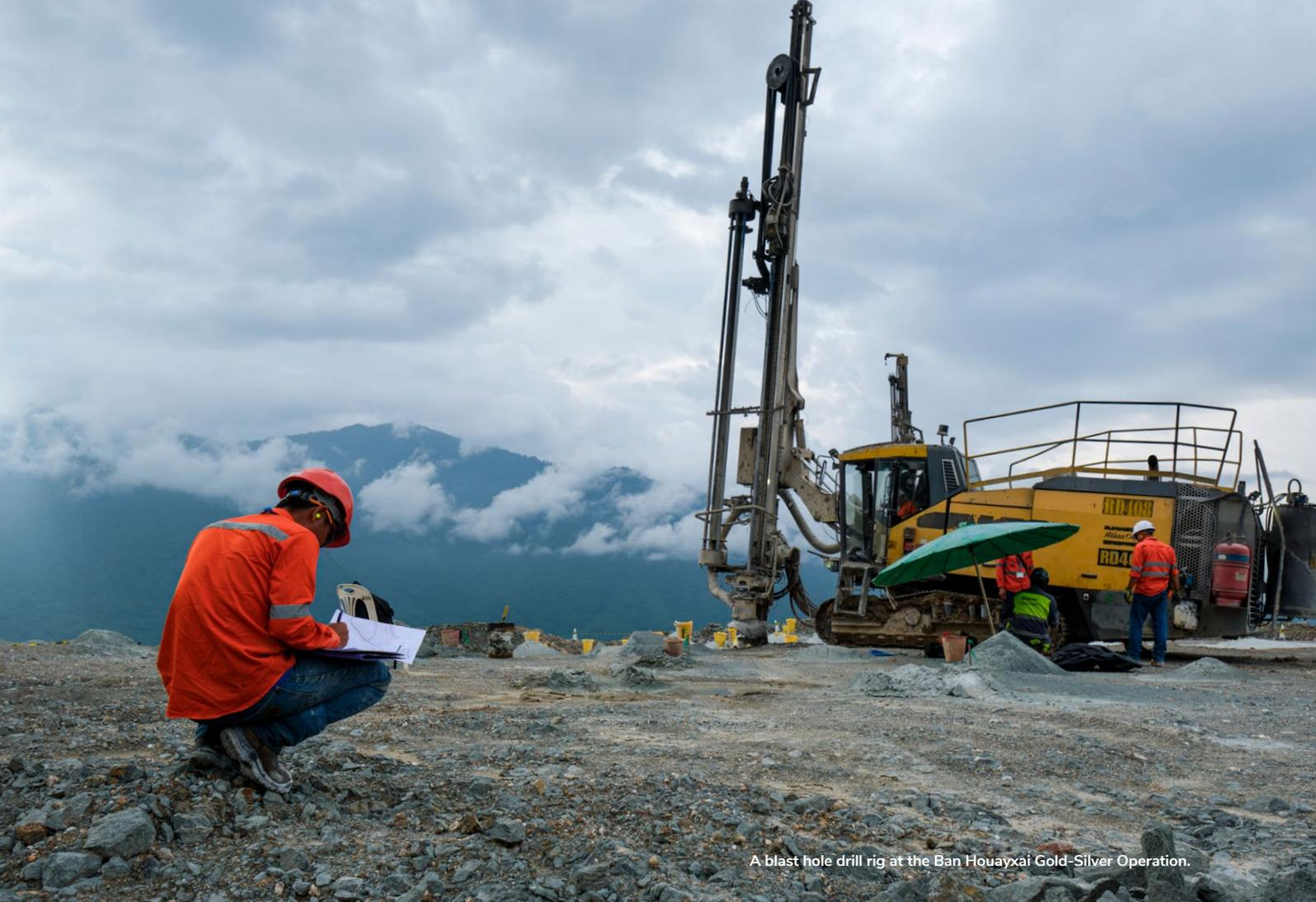
A blast hole drill rig at the Ban Houayxai Gold-Silver Operation.
