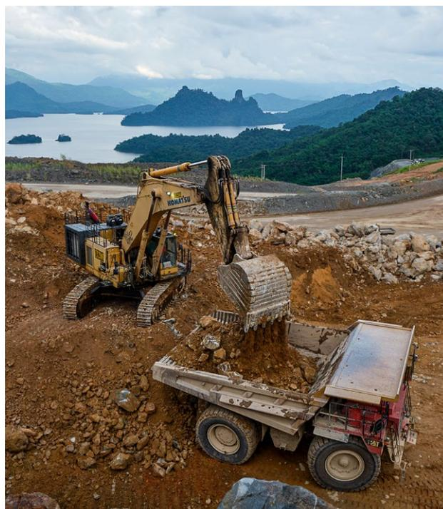
Cat® 777D—100 tonne rigid chassis dump truck being loaded at the Ban Houayxai Gold-Silver Operation.
