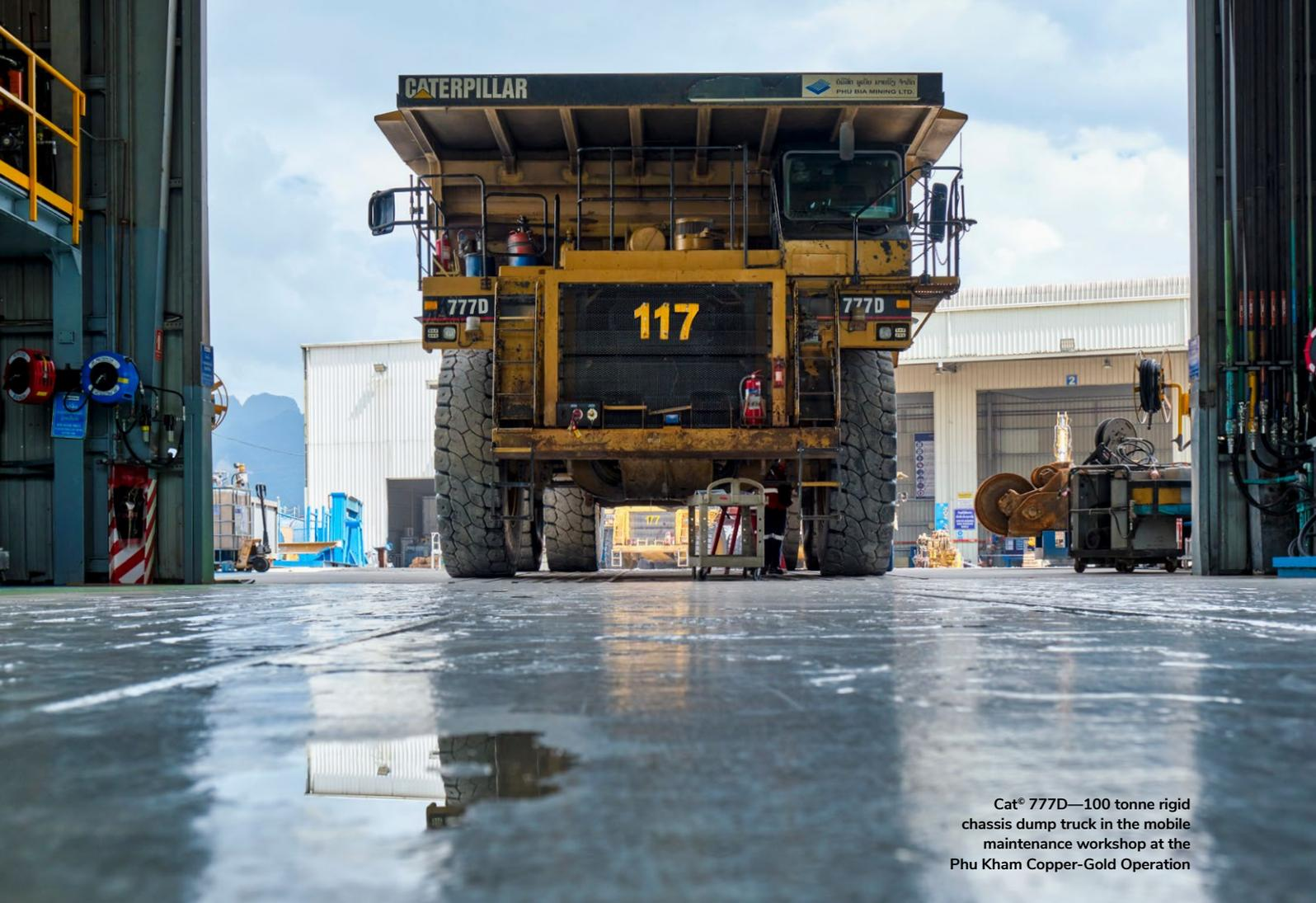
Cat® 777D—100 tonne rigid chassis dump truck in the mobile maintenance workshop at the Phu Kham Copper-Gold Operation
