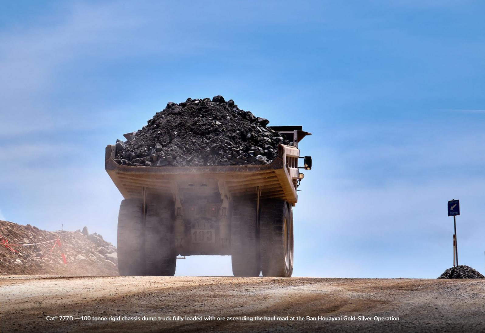
Cat® 777D —100 tonne rigid chassis dump truck fully loaded with ore ascending the haul road at the Ban Houayxai Gold-Silver Operation
