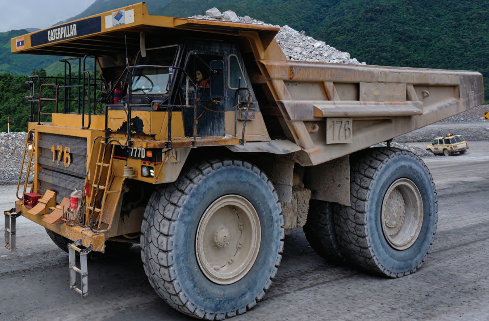
Cat® 777D – 100 tonne rigid chassis dump truck fully loaded with ore ascending the haul ramp at the Phu Kham Copper-Gold Operation
