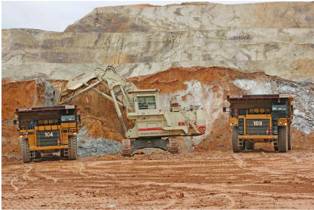
Double sided loading at Phu Kham Operations; a key productivity improvement
