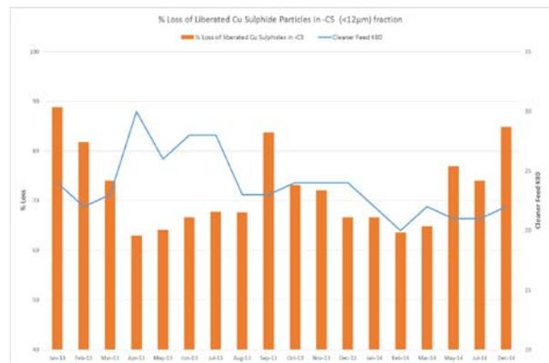
**FIGURE 4 Percent loss of liberated Cu in the -C5 fraction of cleaner tailings**
