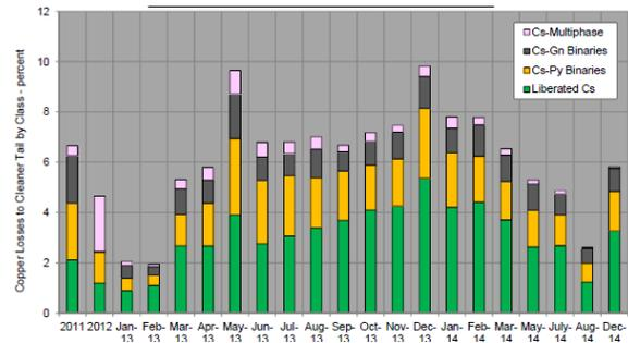
**FIGURE 3 Trend of Cu loss distribution to cleaner tailings by class from mineralogical analysis**
