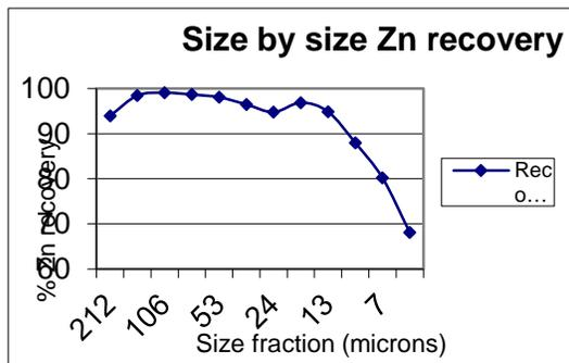
**FIGURE 5 Zinc flotation recovery by size at Golden Grove**
