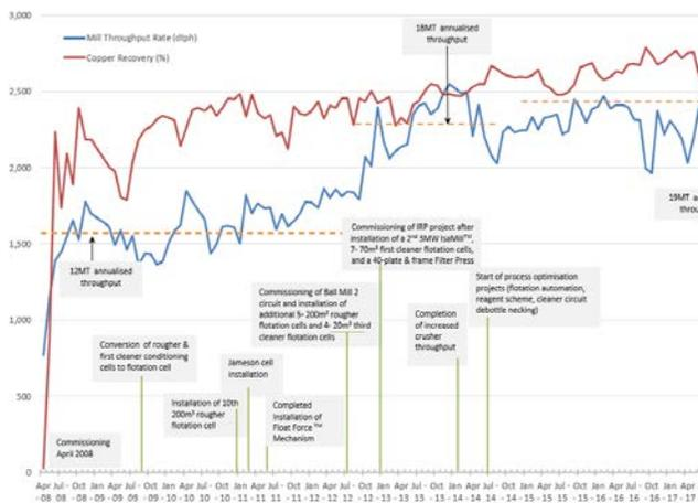
**FIGURE 2 PKO development milestones with throughput and Cu recovery performance**
