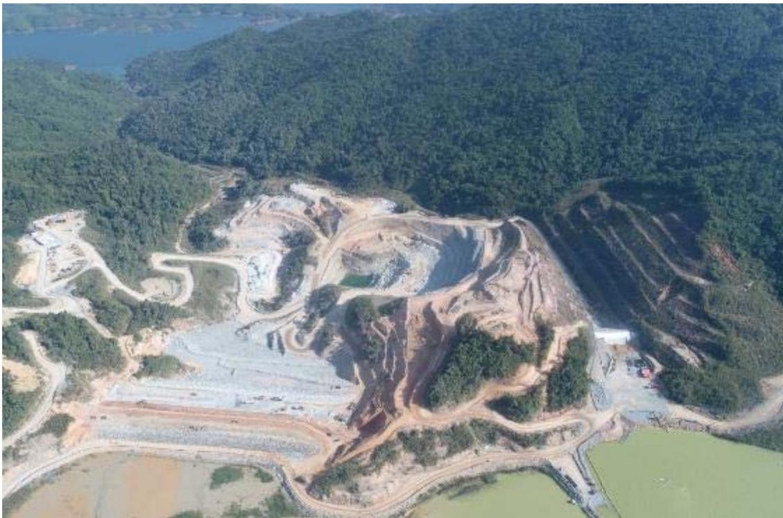
FIGURE 3 - Ban Houayxai TSF embankment, construction quarry and spillway with tailings in foreground
