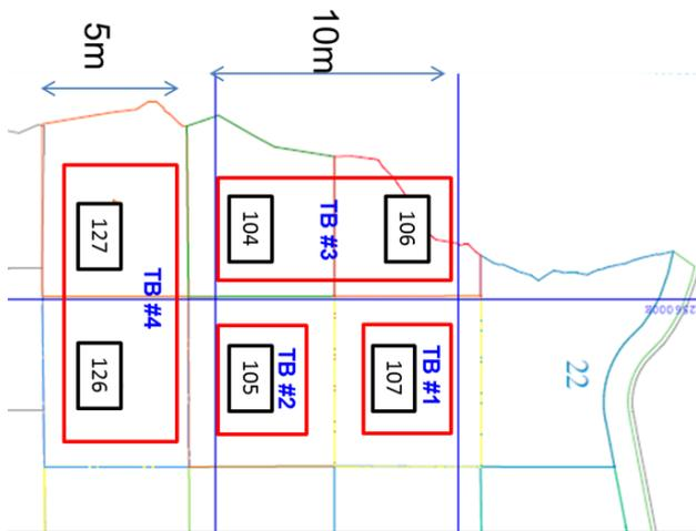
Figure 5. Trial blasts layout
