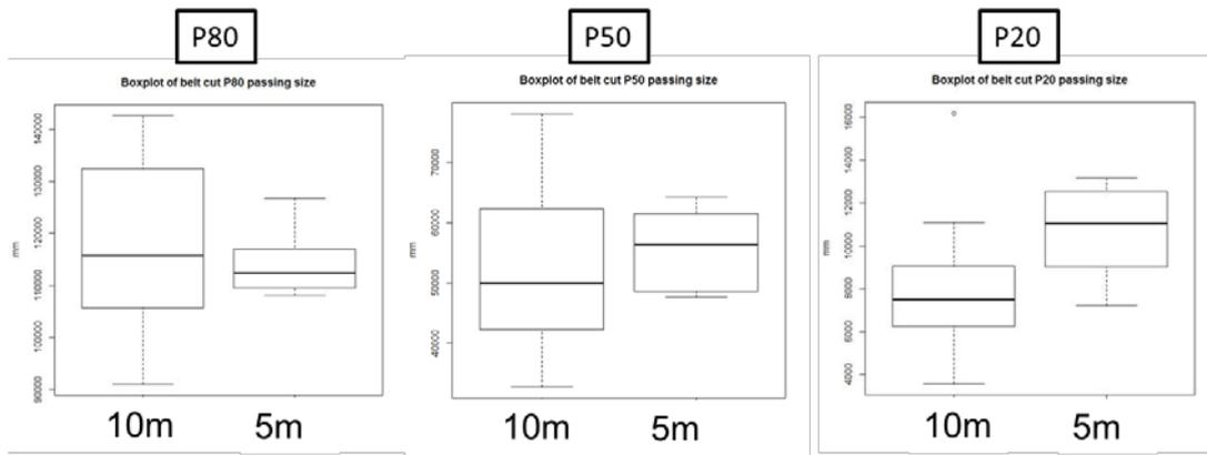
**Figure 7. Size distribution from primary crusher product belt cuts**
