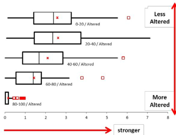
Figure 2 Relationship between point load strength I50 and alteration
