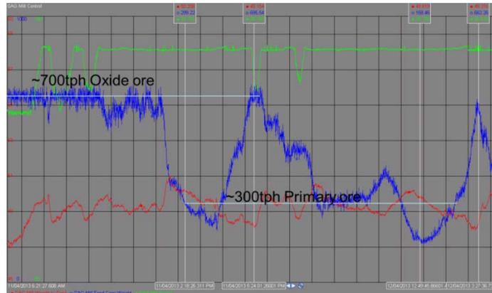
Figure 1. Impact of hard primary ore on SAG mill throughput
