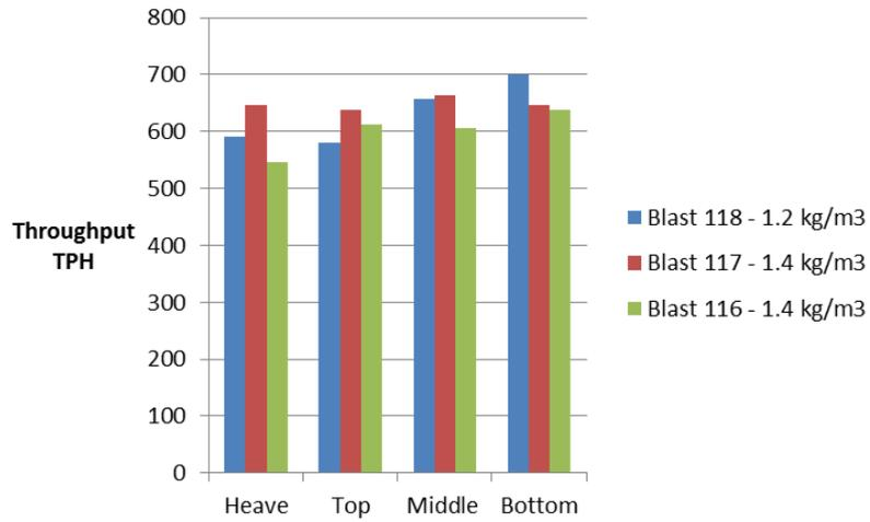
**Figure 10 Median throughputs by flich for the high energy trials**
