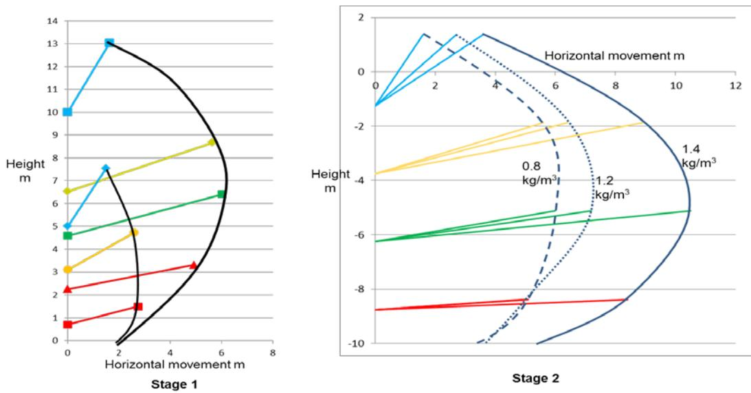
**Figure 11. Measured blast movements from blasting trials from stage 1 and stage 2**
