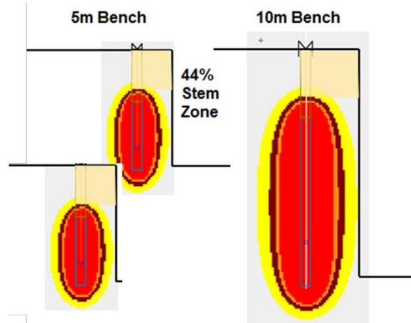
Figure 4. Explosive energy distribution in 5m and 10m Benches
