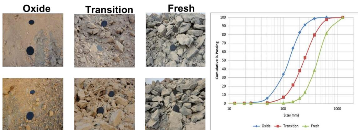
Figure 3 Fragmentation from oxide, transition and primary ores
