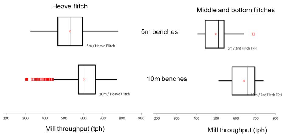
**Figure 8 Mill throughputs for different flitches from 5m and 10m bench blasts**
