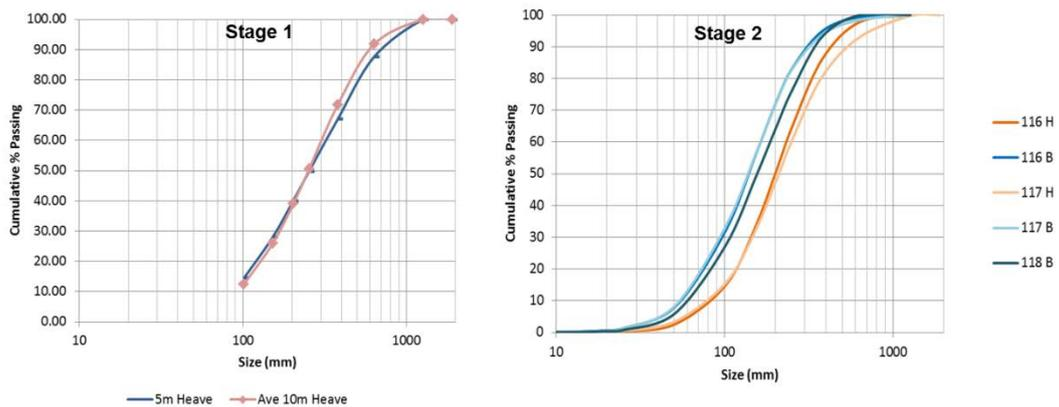
**Figure 9 Fragmentation for heave and bottom flitches FROM STAGE 1 AND 2**
