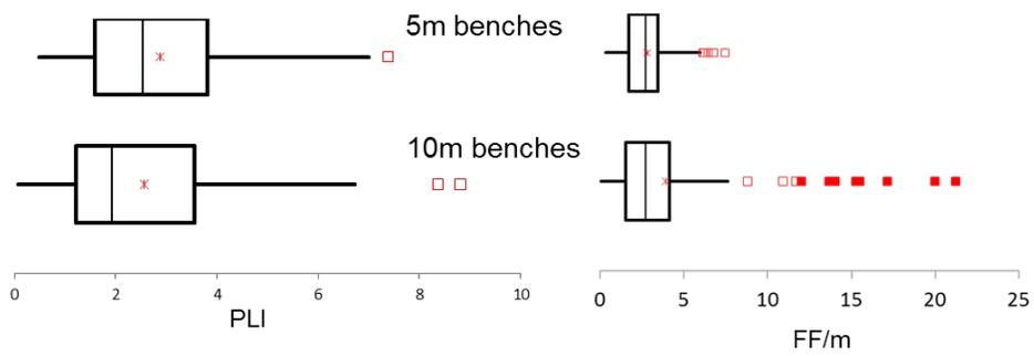
Figure 6. Strength and structural characteristics of ore in 5m and 10m trial blasts
