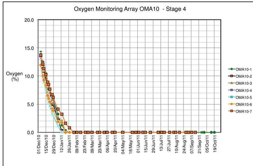
Figure 9. PAF cell pore gas oxygen concentration trends.
