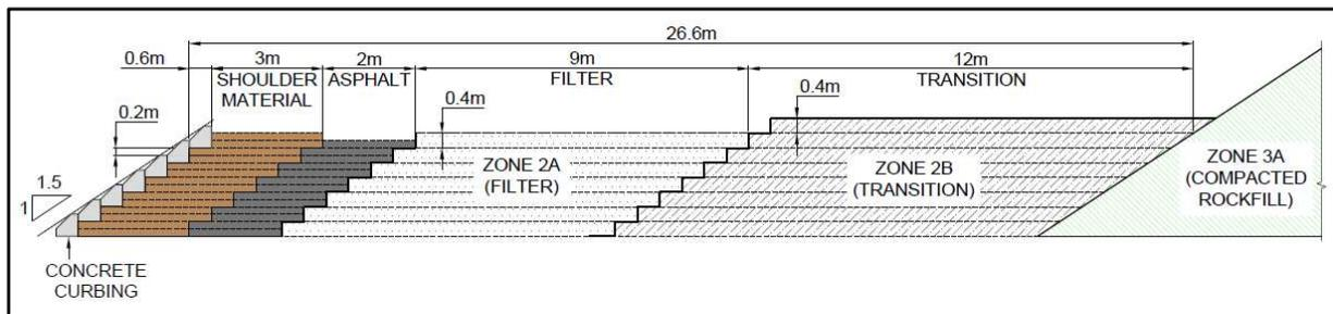
Figure 4 – Upstream inclined core zone
