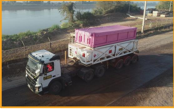
*Left: A truck bound for the Phu Kham Copper-Gold Operation loaded with a full fuel tank (bottom) and an empty concentrate container (top)*
